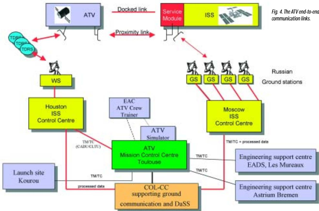
Fig. 4. The ATV end-to-end communication links.
